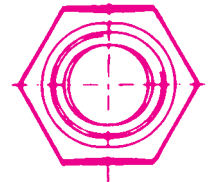
Self-locking conical nut
